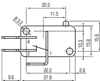
The trip refer to the action of the cam on contact 1-2 (NC)
